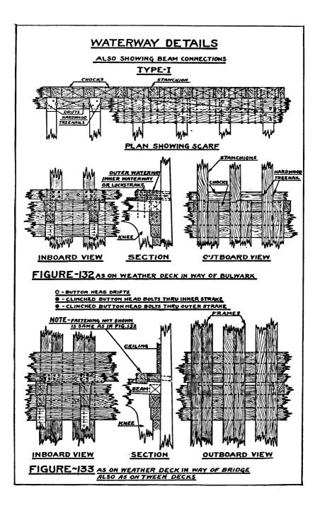
outboard face. The calking seam for the inboard face is generally run on the waterway strake.
