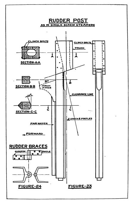
Very often the main piece of this post is made of hardwood. A fairwater is fitted on the forward side of all rudder posts, as shown in Fig. 23. This is spiked in place with ship spikes, after the arch knees have been fitted.
