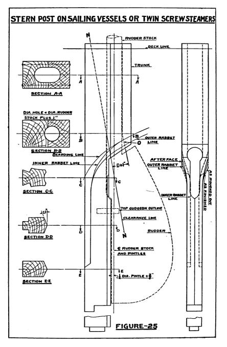
gudgeon. This line is the clearance line, and represents the foremost extent of the hole in the trunk required to clear the stock past the top gudgeon when shipping the rudder.
