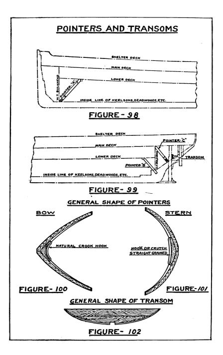
end should land exactly on one of the lines scribed on the ceiling. It will be seen that the length of the cleats will be the same as the sided dimension of the pointer, or the distance between the two lines, and that the upper mold will be held with its lower face even with the line, while the lower mold will be held with its upper face even with the line. Each mold should be scribed on the face that is even with the line.
