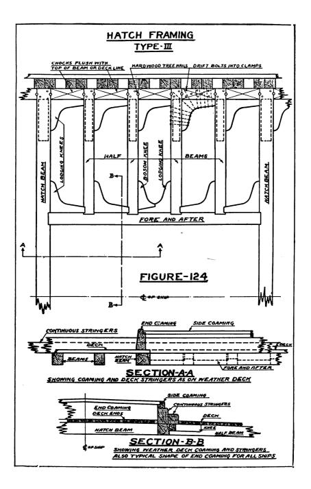
treenail set in the joint between beam and chock at each end to assist in locking the beam in place. In some cases the chocks are omitted in way of the lodging knees, the latter then being fitted direct to the frame. Where this is done and the beam spacing is the same as that of the frames with a beam against each frame, the bays must be chocked to provide room for driving sufficient knee fastening.
