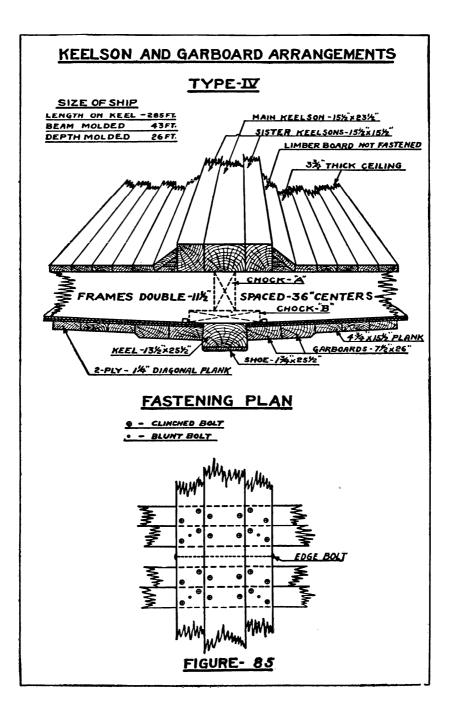
below. In both systems the sister keelsons are edge bolted, it being generally customary to drive the bolts through and clinch them. Their number and arrangement may vary somewhat in different vessels, as also may the other fastening. In all cases detail plans are furnished, showing the exact arrangement of the fastening, and should be carefully followed.
