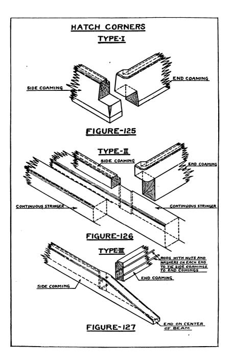
rabbet is also cut across the corner at an angle of 45 degrees. Note that this coaming is not beveled off on the outer face below the top of the continuous stringer as this would make it very difficult to fit in the dap.
