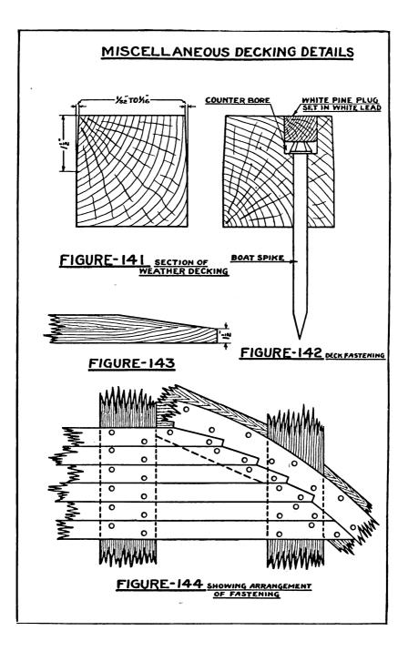
the spike is set down snug there will be from  ${}^{5}/{}_{8}$  to  ${}^{3}/{}_{4}$  inch of depth left for the plug. The plugs are then dipped in thick white lead and tapped down against the spike head. They should fit tight in the counterbores.
