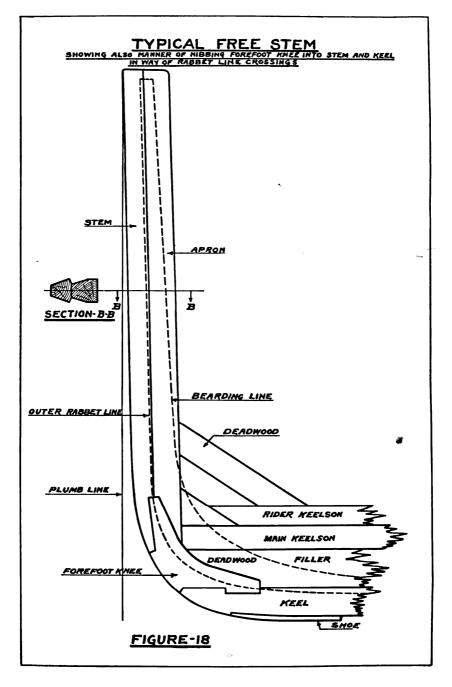
together on the ground. If knightheads are fitted they are also worked out and fastened down to the apron at this time. (Knightheads are really a part of the frame and will be more fully described in the next chapter on framing.) Then, at the proper time, the entire stem structure is erected and shored in position. Three long, heavy shores are used—one forward and one on each side. Care must be taken to set the stem plumb and to the correct rake with the keel.
