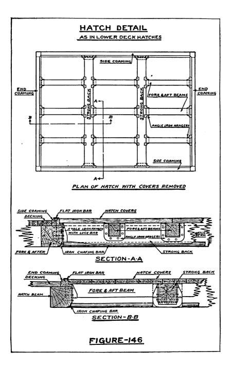
In Fig. 146, due to the smaller depth of the hatch, the beams and strongbacks must be set in the same line and all are supported by means of angle iron hangers. Here the fore and aft beams are not continuous but are cut in between the strongbacks. It should also be noted that the toes of the hangers are turned over at the top to furnish additional bearing to that given by the fastening, and that in addition to this the hangers for the strongbacks have one lock bar.
