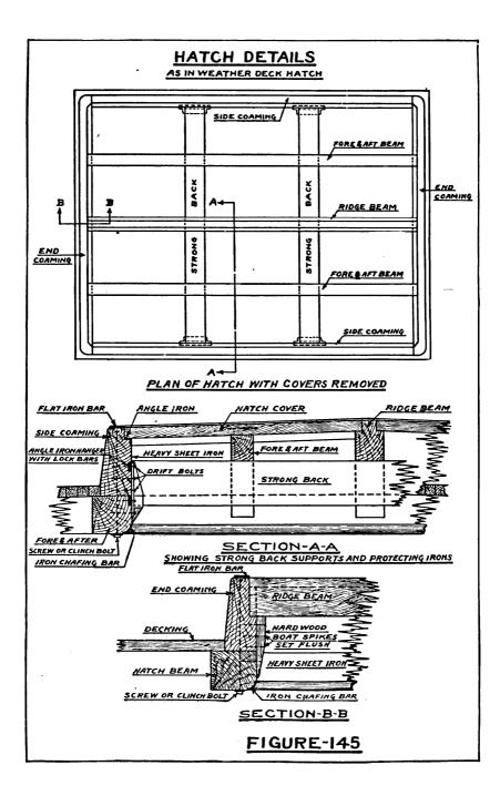
be taken aboard in a heavy sea, according to whether or not a deck load is carried. This requirement that the covers be strong enough to carry heavy loads, necessitates, in the case of large hatches such as cargo hatches, the fitting of a removable system of beams under the covers, one type of which has been detailed in Figs. 145 and 146.
