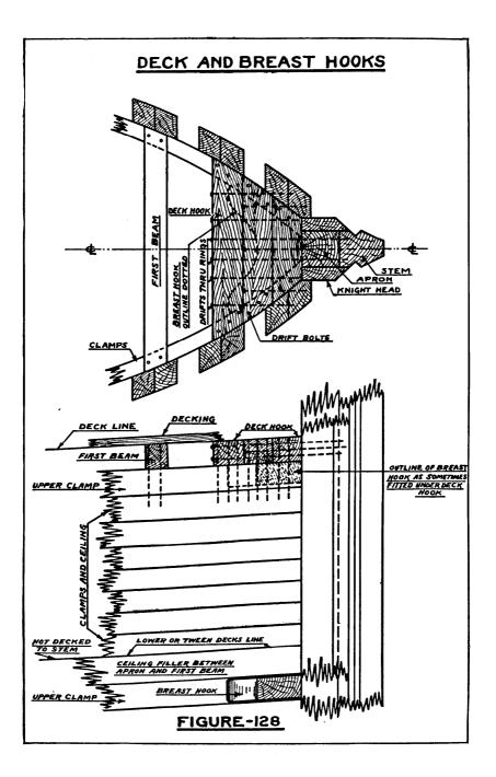
Where care is exercised the timbers forming the hook may be worked to the deck camber before being placed but it is generally best to leave them a little high so that they may be dubbed to the correct camber after being fastened down. To allow for necessary dubbing the bolts fastening the deck hook to the clamps are often plain drifts set in. Where they are button-headed bolts, or plain-headed bolts driven through rings, they should be counterbored and set in.
