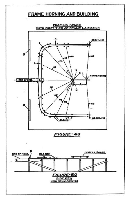
H1, H2, H3, and H4 represent horning diagonals, and these may or may not remain in the same relative position. In square frames forward and aft it is sometimes advisable to carry the horning points further up on the frame, but if the horning points are properly marked on the timbers this will not change the system of horning, or cause confusion.
