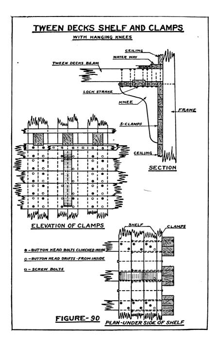
if the lower leg of the knee in Fig. 90 had eight through fastenings, then it would be possible to omit that number of fastenings from the clamps in way of the knee.
