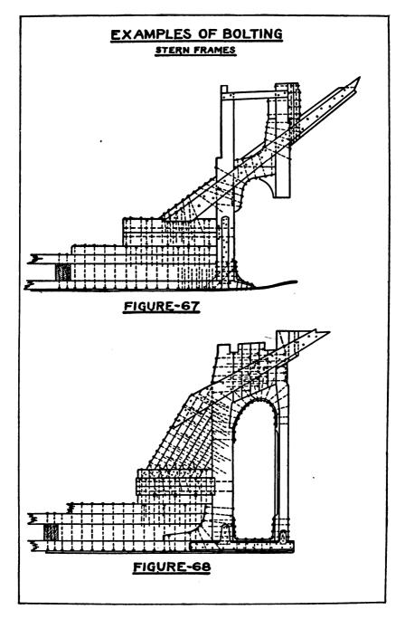
of the propeller-post and fillers show cuts in way of deck beams so that they may be carried through from side to side in one piece. The sterns of these vessels above the rim are generally built up of solid work, as indicated in the figure. Some have been built with radial frames extending up from the rim and mortised into the same, but this construction is somewhat weaker than that obtained with the solid work.
