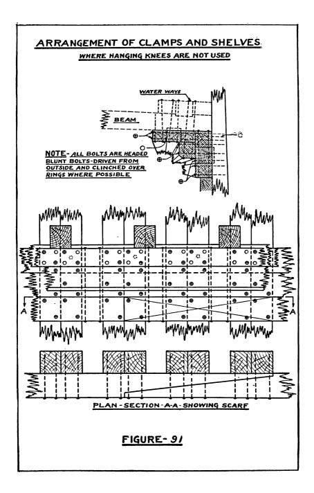
and is clinched below. The shelves are also fastened horizontally into the frame, as are also the waterways, although the bolts are not shown in this figure. It will be readily seen that in order to secure the best job the waterways and shelves should be run in at the same time so the fastening each way in each strake can all be driven, thus securing and holding the strake "home."
