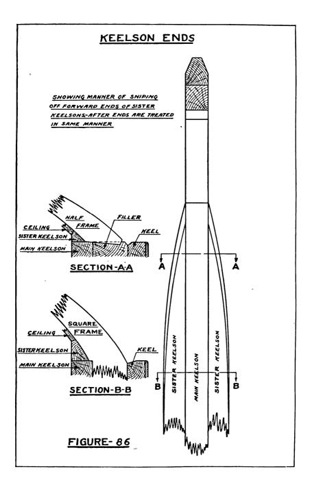
keelsons forward and aft are sniped off to fay to the edges of the ceiling coming in contact with them at that point. This is accomplished in the manner shown in Fig. 86. The ends of the sister keelsons may be worked out from offsets furnished from the loft, these being carefully checked from the ship before cutting the timbers to exact size.
