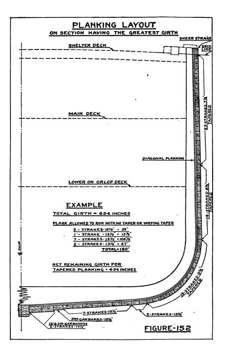
belt of tapered planking at the two points may be quickly estimated.
