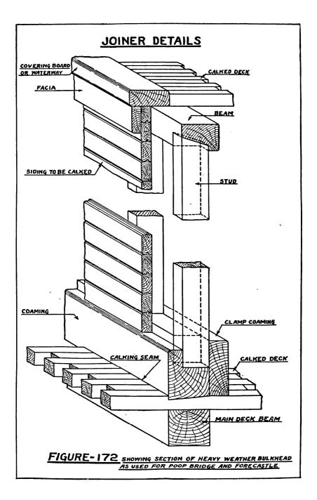
This arrangement, while giving a better calking seam, weakens the decking and is therefore open to objection.
