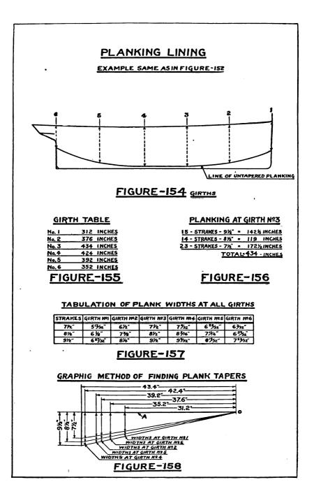
find the required width at any other girth less than the greatest girth it is only necessary to find the percentage that the lesser girth bears to the greatest girth, then this same percentage of the width of the strake at the greatest girth will give the required width at the lesser girth. This operation may be set down as follows:
