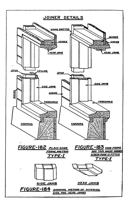
on top of the threshold, and the entire frame is frequently built in the joiner shop and set in place as a unit.
