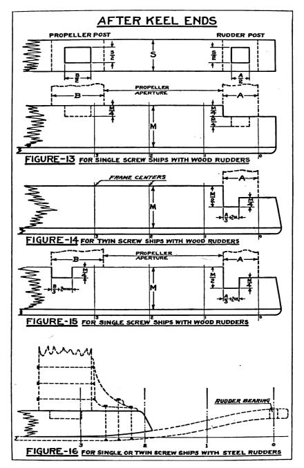
post is also the stern post. See Figs. 13 and 15. A singlescrew ship with a steel rudder will have propeller post, which is also the stern post. See Fig. 16. A twin-screw ship, with a wood rudder, will have a stern post, which is also the rudder post, and will have no propeller post. See Fig. 14.
