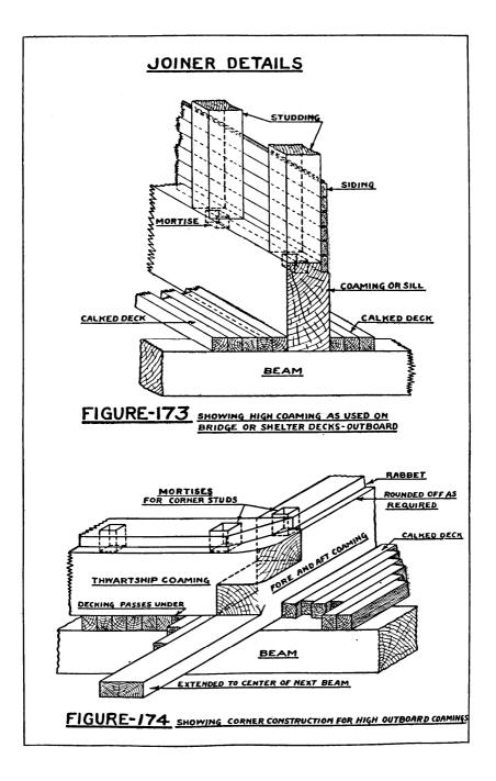
springing must be scribed from wider timber to the shape, or camber, of the deck. All coamings, whether on calked or joiner decks, should be thoroughly fastened with either screw or clinched bolts, preferably the former, passing through the beams, with nuts set up below on large washers.
