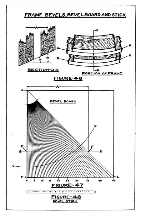
point between the lines M-M and N-N, and X the angle which it is desired to find, by measuring the distance B.
