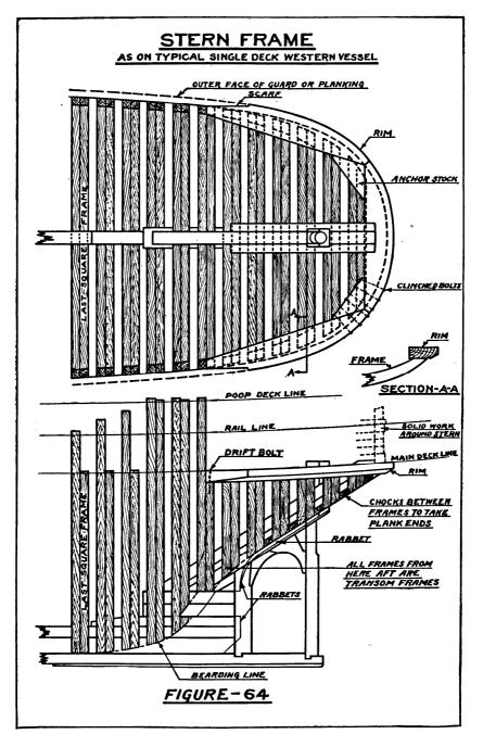
The poop erection on these vessels is often very short, and forward of same, in way of the bulwark, but one-half of the frame, that is, the stanchion, is carried above the deck, as shown in Fig. 64.
