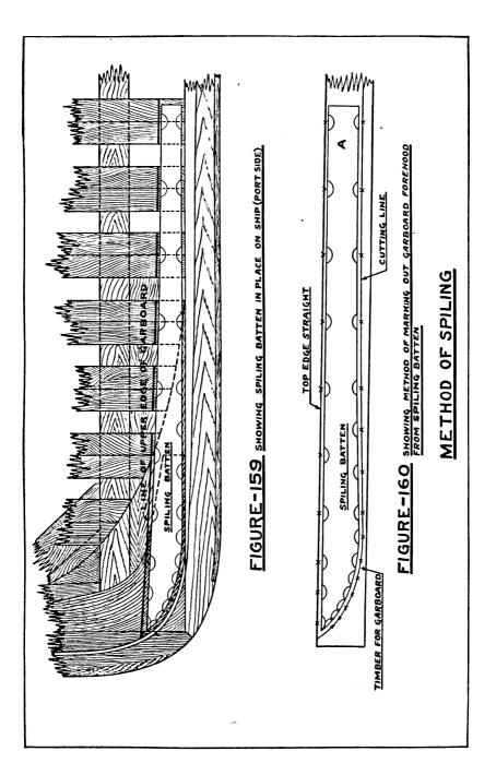
of the timber. The balance of the points are then marked off with the batten held in this position. It will thus be seen that with the same spiling batten, it is possible to lay out the garboard forehood with either no edge set, or the full edge set required by leaving the upper edge of the garboard straight, or any intermediate desired edge set, according to the conditions, width of available stock, and the liners judgment.
