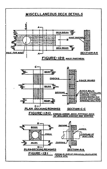
The bolts fastening the partners should pass through beam and beam and be clinched over rings on each end. Sometimes an end chock, dapped into the beams, is fitted as shown by the dotted outline at "B," but this is rather unusual in steamers.
