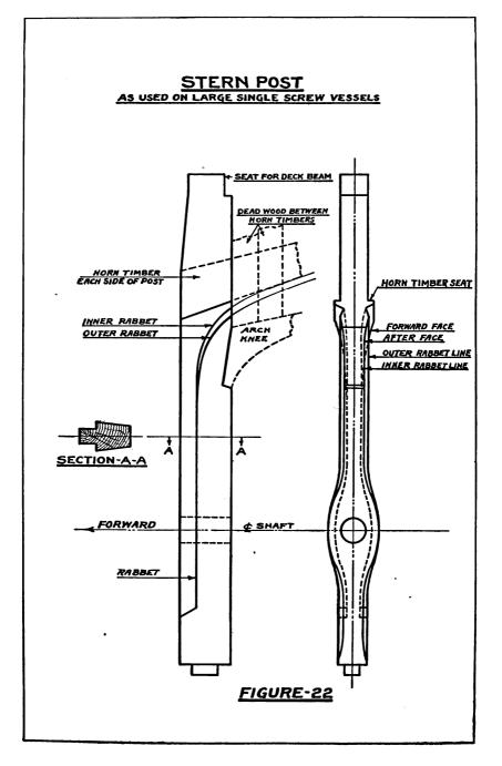
lay them out with sufficient accuracy. But the shape of the post, in siding, can, and ought to be, roughed out a little over size, as this saves dubbing after erection. The post is not finally faired off to the shape shown in the figures until after the planking has been completed.
