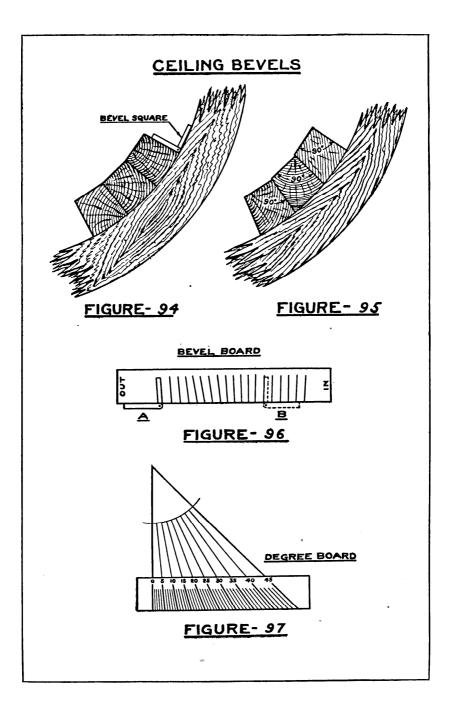
bevel board. It is not always necessary to number them. If they are taken, say at every other frame, and in order, then it is only necessary for the bevel taker to remember where he started taking the bevels.
