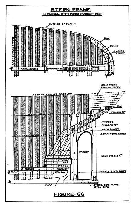
A small rim is fitted inside the cants with its top face on the deck line, to receive the ends of the decking.
